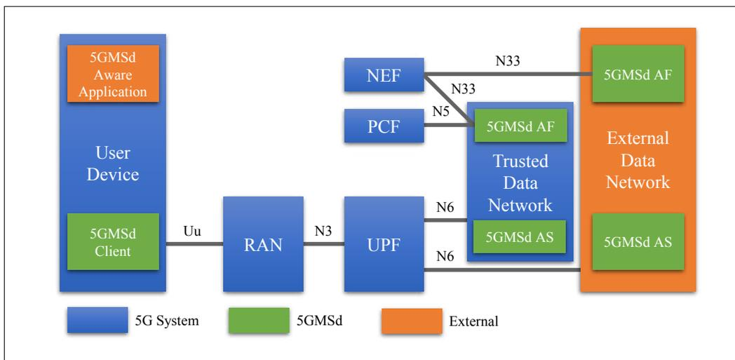
Figure 2. 5G Media Downlink Streaming (5GMSd) for the 5G System [7]. NEF (Network Exposure Function), PCF (Policy Control Function), UPF (User Plane Function) are network functions of the 5G System. AF (Application Function) and AS (Application Server) are defined by the 5GMSd.
