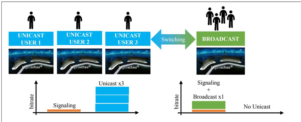
Figure 3. Simplification of the Dynamic switching between unicast and broadcast according to increasing audience demand
